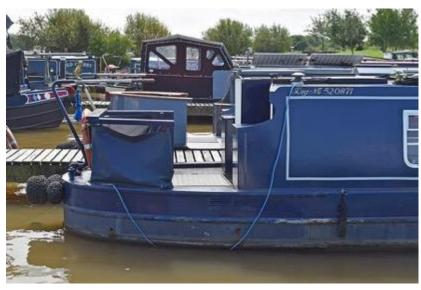
Steel rear doors, wood panelled internally with sliding roof hatch lead to the cruiser deck and steering position.
