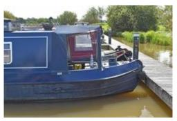
From the bow which has a storage locker, there is a 4' self draining well deck. There is a cratch frame with window to the front and a vinyl cover and a 12v wall light. The stainless steel water tank is located beneath the well deck with a surface mounted filler.
