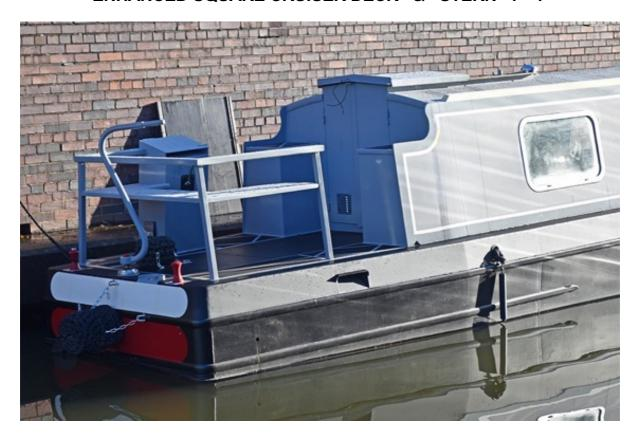
Steel rear doors with sliding roof hatch lead onto the cruiser deck and steering position. There are lift up access panels to the engine and batteries. Lockers to either side of the rear doors.
