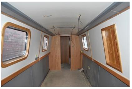
Lined internally with grey and white melamine panels and solid oak trims, including mushroom vent liners, window and door liners. Two full height bulkheads, to allow for a reverse layout with walk through bathroom
