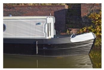
From the bow which holds the steel storage locker, there is a 3 '8" open self draining well deck. The water tank is located beneath the well deck with a surface mounted filler. The headlamp is mounted on the front bulkhead.
