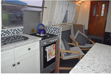
**Appliances:** New Statesman slot in gas cooker with a lid/splash-back. New 12v, essentials fridge with freezer compartment. Ecoplus gas fired instant water heater. Inset, sink with integral drainer and glass cover.
