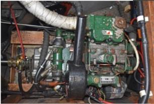
**Controls:** The single lever engine control is on the port side just inside the rear doors.
