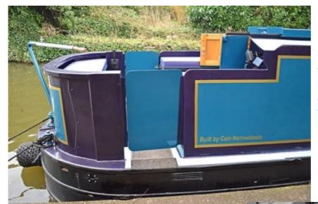
Steel rear doors, wood panelled internally with sliding roof hatch lead to the cruiser deck and steering position.
