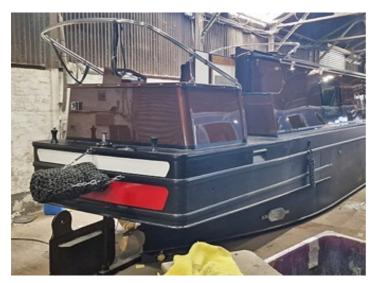
Steel rear doors painted wood panelled internally with sliding roof hatch lead onto the square cruiser deck and steering position. The seating in the enhanced cruiser stern is supplied with padded cushions. There are lift up access panels to the engine and batteries. Gas lockers to either side of the rear doors. Unique design pram cover.
