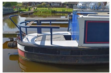
Steel rear doors, wood panelled internally with sliding roof hatch lead to the cruiser deck and steering position.
