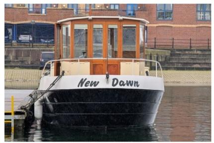
A hardwood door leads from the galley up to the wheelhouse. The glazed mahogany wheelhouse is fully collapsible. The engine room is below the wheelhouse and accessed through the lift up floor panels. Part glazed, side and rear doors lead out to the decks.
