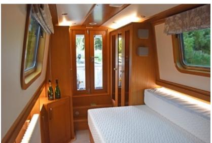
**Lighting:** 2x 3' double glazed top opening windows. 8x 12v LED ceiling lights. 4 x 12v LED under gunwale strip lights. 2 x 12v LED strip lights above the wardrobes.
